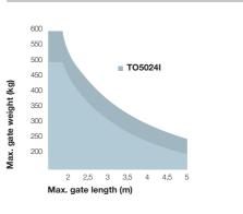
The shape, the height of the gate and the weather conditions can considerably reduce the values shown in the graph to the side. Use in windy areas 230 Vac models.
